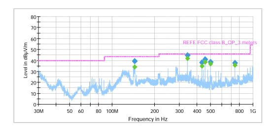
Note: The Blue Markers on the above plots are Peak detectors and are included for information purposes only, EN55032:2015\* requires only the Quasi-Peak detector (Green Markers) in this frequency range to meet the specification limit represented. The marker details are included in table format below.
