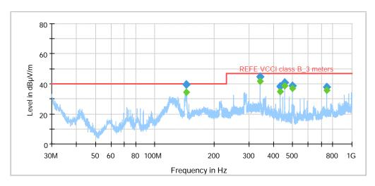
Note: The Blue Markers on the above plots are Peak detectors and are included for information purposes only, EN55032:2015\* requires only the Quasi-Peak detector (Green Markers) in this frequency range to meet the specification limit represented. The marker details are included in table format below.
