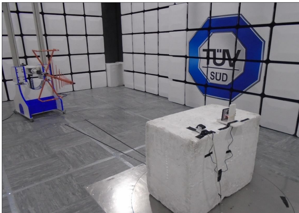
Figure 12 –Test Setup - Below 1 GHz
